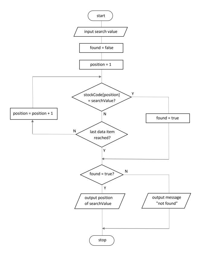
The final step is to output the position in the table where the required stock code was found, or give a message that the stock code was not found.
